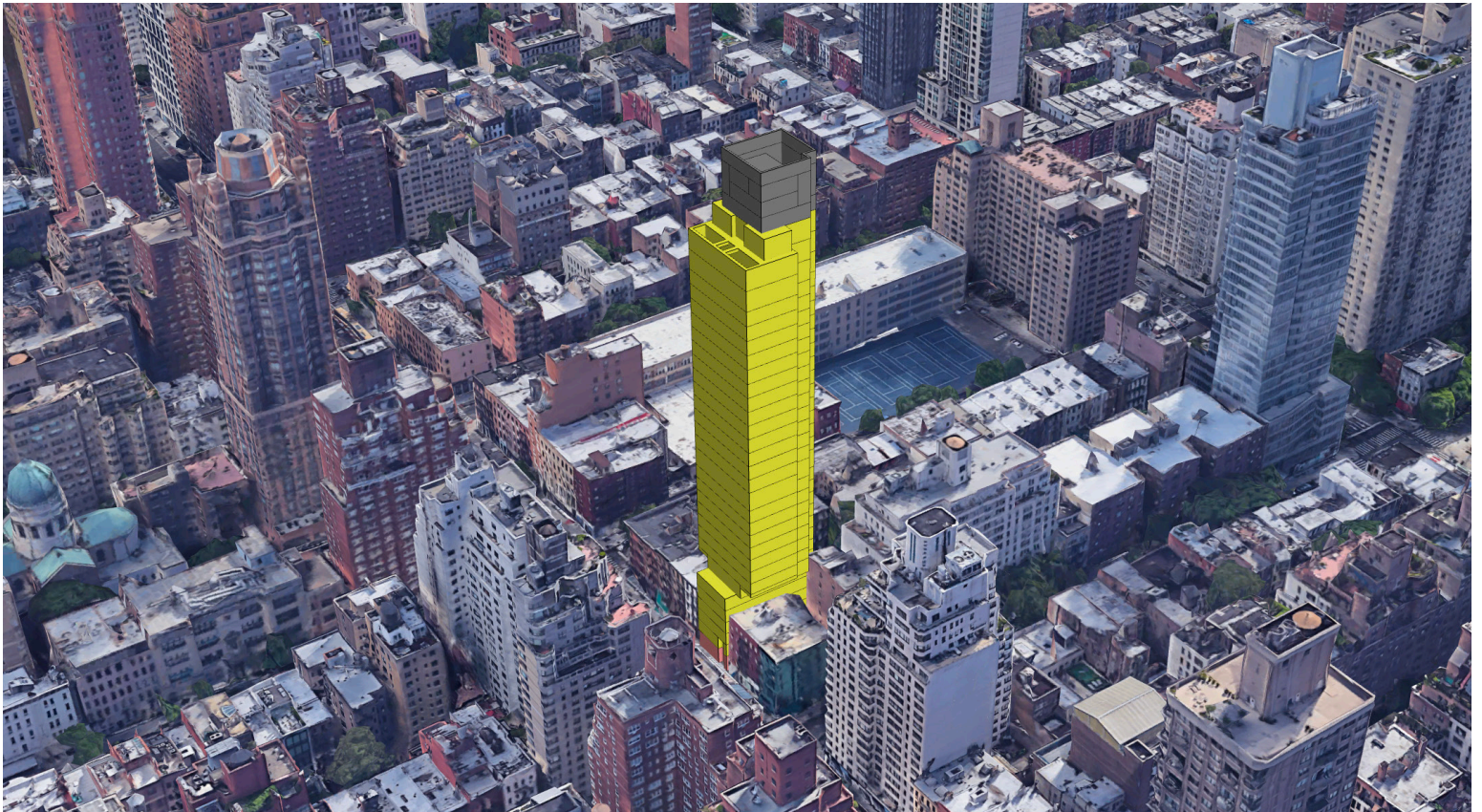
Current zoning approvals indicate a narrow, 33-story residential tower with significant cantilevers over neighboring buildings. Cantilevers of 12 feet to the north and 19 feet to the south allow the tower to be 78% wider than it would be otherwise.
